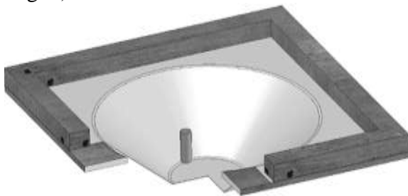
Fig. 1. Single Point Incremental Sheet Forming
