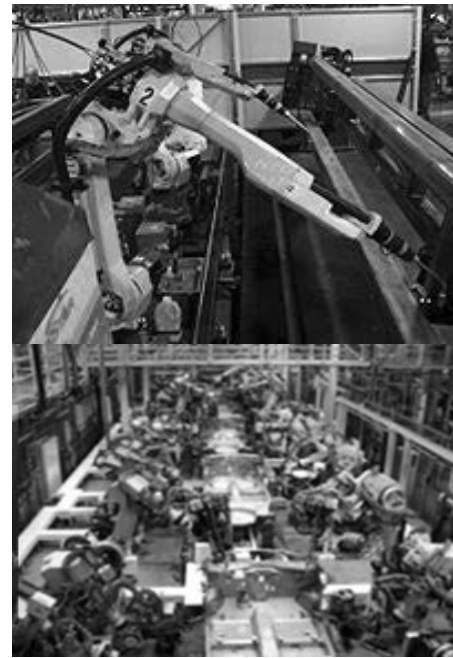
Fig. 6a. Industrial robots – welding application
